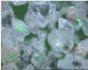
Figure 31| Silicon on ferrogram [37]
