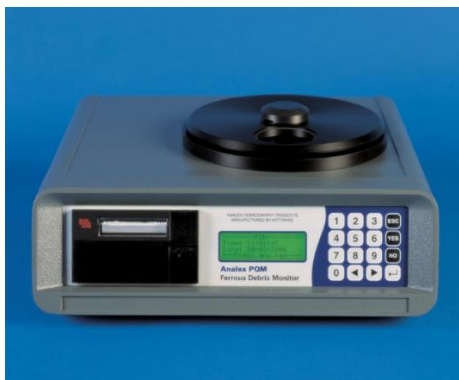
Figure 12| Analex PQA Ferrous Debris Monitor
