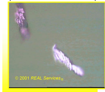
Figure 28| Aluminium particle on ferrogram [34]
