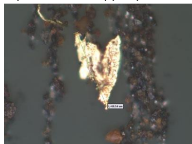
Figure 29| Copper particle on ferrogram [35]
