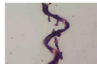
Figure 39| Cutting wear particles [38]
