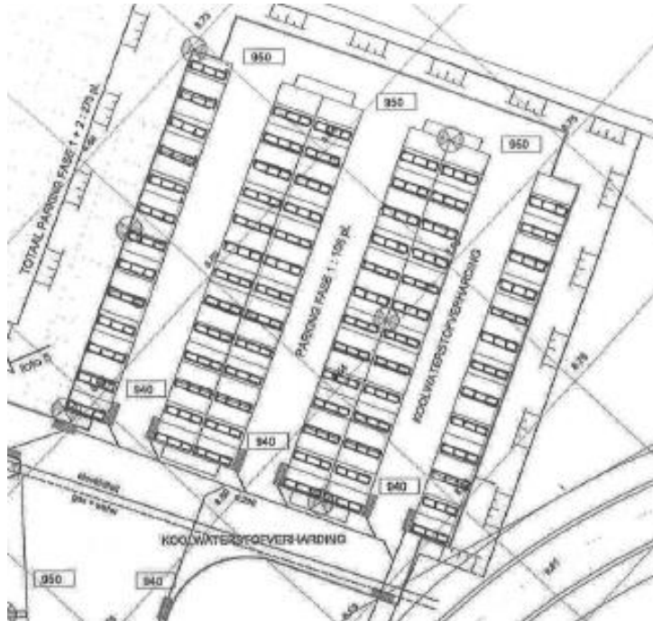
Figure 57: Final location of polycrystalline panels in big parking
