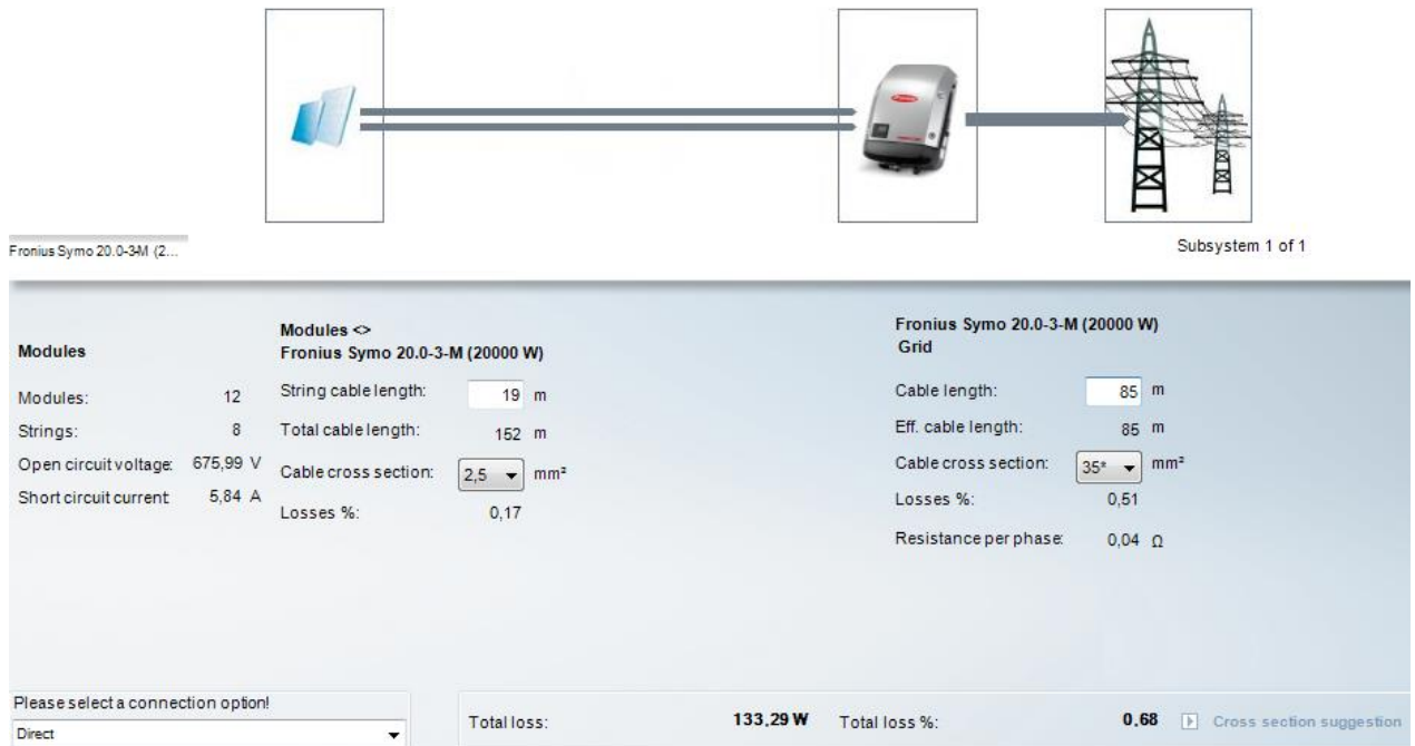
Figure 26: Configuration of the cables
