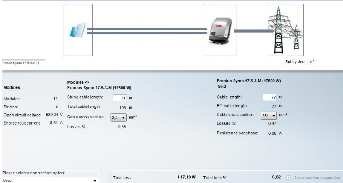
Figure 44: Configuration of the cables
