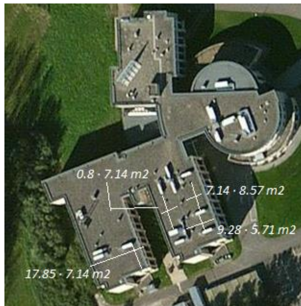
Figure 13: Location of extra surface in the roof
