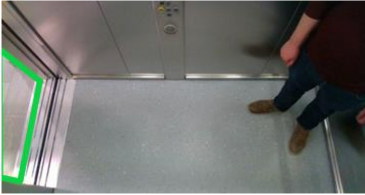
Figure 61 Highlighted detection area
