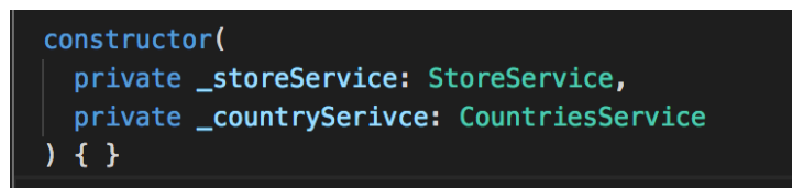
Figuur 16 Inladen services via constructor
